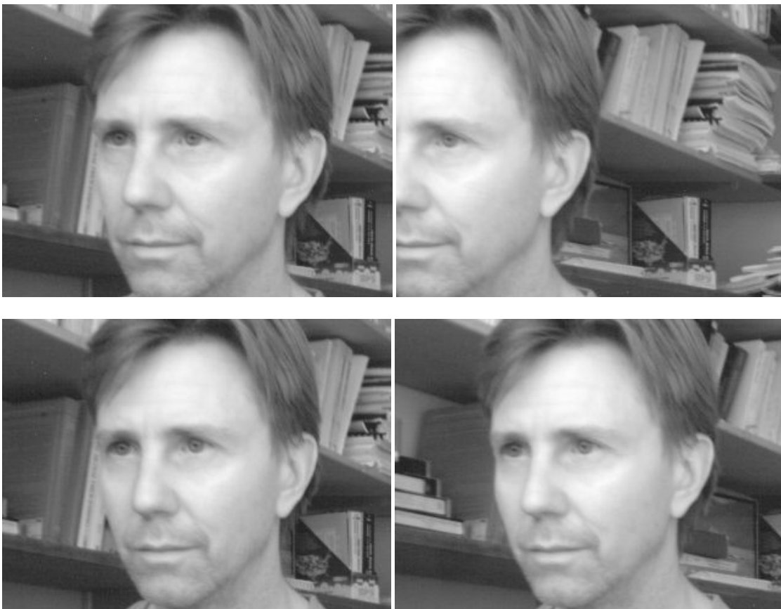
Figure 2-5 Parallel image subwindows (top) and verged image subwindows (bottom), showing a close object.
